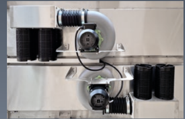
Two powerful fans and four filters on the back
